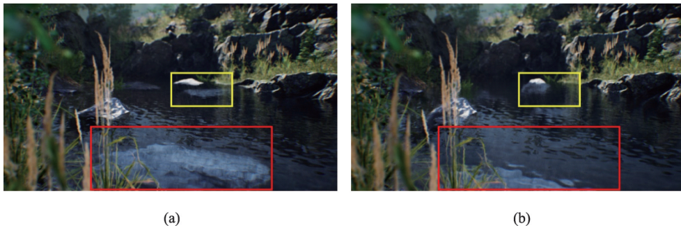
Figure 14 Comparisons of the rendering results of water in an outdoor scene of a video game. (a) The underwater geometries are refracted using our method; (b) The refracted parts are incorrect in the commonly used screen-space approach in most video games.
